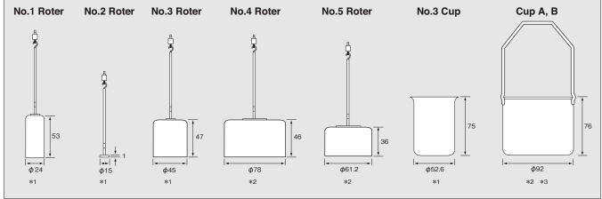
\*1 Material: Stainless steel \*2 Material: Aluminate \*3 Cup B has a 30 mm diameter hole at the bottom. Use Cup B to measure viscosity by directly by dipping Rotor in the fluid.
